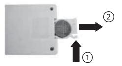
Place the battery in the bracket with the + symbol facing out. When the battery is in the bracket, the + symbol should be visible.
